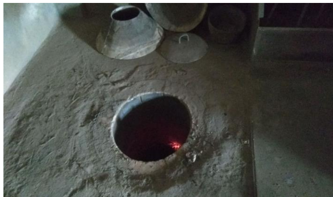
Figure 5: Pit type coal fired furnace
