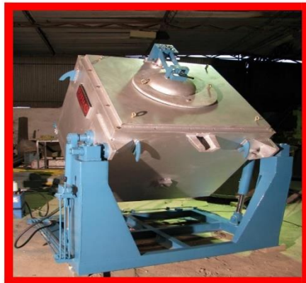
Hydraulic Tilting Furnace
